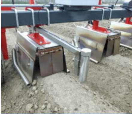
Wind canopy with infrared radiation
